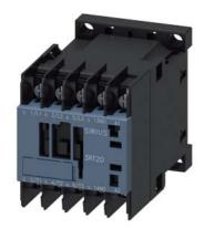
power contactor, AC-3e/AC-3, 9 A, 4 kW / 400 V, 3-pole, 110 V AC, 50 Hz / 120 V, 60 Hz, auxiliary contacts: 1 NO, ring cable lug connection, size: S00
