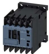
power contactor, AC-3e/AC-3, 9 A, 4 kW / 400 V, 3-pole, 110 V AC, 50 Hz / 120 V, 60 Hz, auxiliary contacts: 1 NC, ring cable lug connection, size: S00  $\,$
