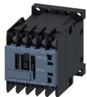
power contactor, AC-3e/AC-3, 9 A, 4 kW / 400 V, 3-pole, 200 V AC, 50 Hz / 200-220 V, 60 Hz, auxiliary contacts: 1 NO, ring cable lug connection, size: S00  $\,$
