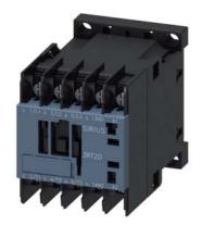
power contactor, AC-3e/AC-3, 9 A, 4 kW / 400 V, 3-pole, 220 V AC, 50 Hz / 240 V, 60 Hz, auxiliary contacts: 1 NO, ring cable lug connection, size: S00
