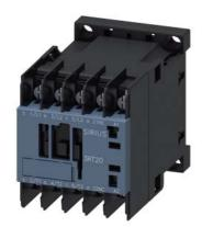
power contactor, AC-3e/AC-3, 9 A, 4 kW / 400 V, 3-pole, 400 V AC, 50 Hz / 400-440 V, 60 Hz, auxiliary contacts: 1 NC, ring cable lug connection, size: S00
