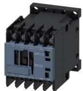
power contactor, AC-3e/AC-3, 9 A, 4 kW / 400 V, 3-pole, 24 V DC, auxiliary contacts: 1 NO, ring cable lug connection, size: S00
