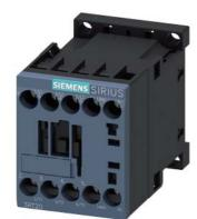
power contactor, AC-3e/AC-3, 12 A, 5.5 kW / 400 V, 3-pole, 24 V AC, 50/60 Hz, auxiliary contacts: 1 NO, screw terminal, size: S00
