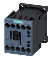
power contactor, AC-3e/AC-3, 12 A, 5.5 kW / 400 V, 3-pole, 110 V AC, 50 Hz / 120 V, 60 Hz, auxiliary contacts: 1 NO, screw terminal, size: S00
