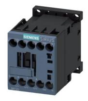
power contactor, AC-3e/AC-3, 12 A, 5.5 kW / 400 V, 3-pole, 110 V AC, 50 Hz / 120 V, 60 Hz, auxiliary contacts: 1 NC, screw terminal, size: S00
