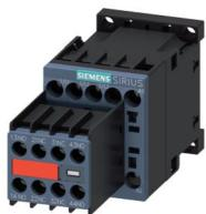
power contactor, AC-3e/AC-3, 12 A, 5.5 kW / 400 V, 3-pole, 110 V AC, 50 Hz / 120 V, 60 Hz, auxiliary contacts: 2 NO + 2 NC, screw terminal, size: S00, captive auxiliary switch
