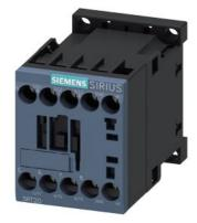
power contactor, AC-3e/AC-3, 12 A, 5.5 kW / 400 V, 3-pole, 208 V AC, 50/60 Hz, auxiliary contacts: 1 NC, screw terminal, size: S00  $\,$
