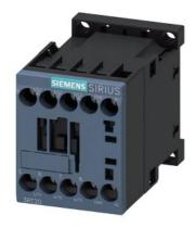
power contactor, AC-3e/AC-3, 12 A, 5.5 kW / 400 V, 3-pole, 220 V AC, 50/60 Hz, auxiliary contacts: 1 NC, screw terminal, size: S00  $\,$
