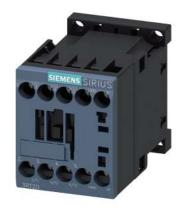
power contactor, AC-3e/AC-3, 12 A, 5.5 kW / 400 V, 3-pole, 230 V AC, 50/60 Hz, auxiliary contacts: 1 NO, screw terminal, size: S00, upright mounting position
