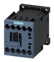
power contactor, AC-3e/AC-3, 12 A, 5.5 kW / 400 V, 3-pole, 230 V AC, 50/60 Hz, auxiliary contacts: 1 NC, screw terminal, size: S00, suspended mounting position
