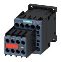
power contactor, AC-3e/AC-3, 12 A,  $5.5\,kW$  /  $400\,V$ , 3-pole,  $230\,V$  AC,  $50/60\,Hz$ , auxiliary contacts: 2 NO + 2 NC, screw terminal, size: S00, captive auxiliary switch
