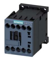
power contactor, AC-3e/AC-3, 12 A, 5.5 kW / 400 V, 3-pole, 220 V AC, 50 Hz / 240 V, 60 Hz, auxiliary contacts: 1 NO, screw terminal, size: S00
