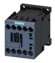
power contactor, AC-3e/AC-3, 12 A, 5.5 kW / 400 V, 3-pole, 600 V AC, 60 Hz, auxiliary contacts: 1 NO, screw terminal, size: S00  $\,$
