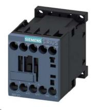
power contactor, AC-3e/AC-3, 12 A, 5.5 kW / 400 V, 3-pole, 24 V DC, auxiliary contacts: 1 NO, screw terminal, size: S00, upright mounting position
