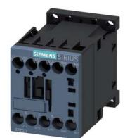
power contactor, AC-3e/AC-3, 12 A, 5.5 kW / 400 V, 3-pole, 24 V DC, auxiliary contacts: 1 NC, screw terminal, size: S00, communication-capable
