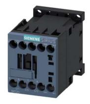
power contactor, AC-3e/AC-3, 12 A, 5.5 kW / 400 V, 3-pole, 230 V DC, auxiliary contacts: 1 NC, screw terminal, size: S00  $\,$
