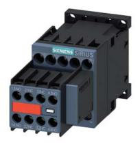
power contactor, AC-3e/AC-3, 12 A, 5.5 kW / 400 V, 3-pole, 110 V AC, 50 Hz / 120 V, 60 Hz, with varistor plugged on, auxiliary contacts: 2 NO + 2 NC, screw terminal, size: S00, captive auxiliary switch
