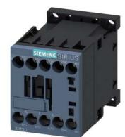
power contactor, AC-3e/AC-3, 12 A, 5.5 kW / 400 V, 3-pole, 24 V DC, with integrated diode, auxiliary contacts: 1 NC, screw terminal, size: S00  $\,$
