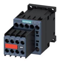
power contactor, AC-3e/AC-3, 12 A, 5.5 kW / 400 V, 3-pole, 24 V DC, with integrated diode, auxiliary contacts: 2 NO + 2 NC, screw terminal, size: S00, captive auxiliary switch
