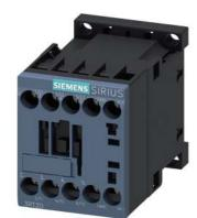
power contactor, AC-3e/AC-3, 12 A, 5.5 kW / 400 V, 3-pole, 12 V DC, 0.7-1.25\* US, auxiliary contacts: 1 NO, screw terminal, frame size: S00, not expandable with auxiliary switch
