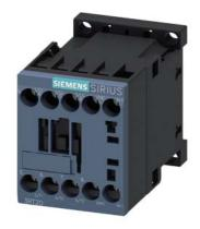
power contactor, AC-3e/AC-3, 12 A, 5.5 kW / 400 V, 3-pole, 24 V DC, 0.7-1.25\* Us, with integrated diode, auxiliary contacts: 1 NC, screw terminal, size: S00, suitable for PLC outputs, not expandable with auxiliary switch
