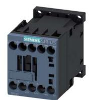
power contactor, AC-3e/AC-3, 12 A, 5.5 kW / 400 V, 3-pole, 24 V DC, 0.7-1.25\* Us, with integrated suppressor diode, auxiliary contacts: 1 NO, screw terminal, size: S00, suitable for PLC outputs, not expandable with auxiliary switch
