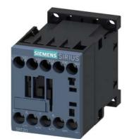
power contactor, AC-3e/AC-3, 12 A, 5.5 kW / 400 V, 3-pole, 24 V DC, 0.85-1.85\* Us, with integrated suppressor diode, auxiliary contacts: 1 NC, screw terminal, size: S00
