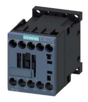
power contactor, AC-3e/AC-3, 12 A, 5.5 kW / 400 V, 3-pole, 24 V DC, with integrated varistor, auxiliary contacts: 1 NO, screw terminal, size: S00, upright mounting position
