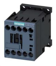
power contactor, AC-3e/AC-3, 12 A, 5.5 kW / 400 V, 3-pole, 24 V DC, with integrated varistor, auxiliary contacts: 1 NC, screw terminal, size: S00, upright mounting position
