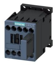
power contactor, AC-3e/AC-3, 12 A, 5.5 kW / 400 V, 3-pole, 24 V DC, 0.85-1.85  $^{\star}$  Us, with varistor plugged on, auxiliary contacts: 1 NC, screw terminal, size: S00, not expandable with auxiliary switch
