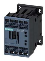
power contactor, AC-3e/AC-3, 12 A, 5.5 kW / 400 V, 3-pole, 24 V AC, 50/60 Hz, auxiliary contacts: 1 NO, spring-loaded terminal, size: S00, upright mounting position
