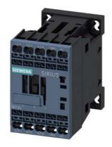
power contactor, AC-3e/AC-3, 12 A, 5.5 kW / 400 V, 3-pole, 24 V AC, 50/60 Hz, auxiliary contacts: 1 NO, spring-loaded terminal, size: S00
