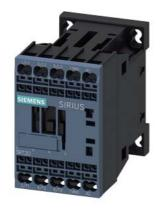
power contactor, AC-3e/AC-3, 12 A, 5.5 kW / 400 V, 3-pole, 110 V AC, 50/60 Hz, auxiliary contacts: 1 NO, spring-loaded terminal, size: S00
