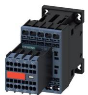
power contactor, AC-3e/AC-3, 12 A, 5.5 kW / 400 V, 3-pole, 110 V AC, 50 Hz / 120 V, 60 Hz, auxiliary contacts: 2 NO + 2 NC, spring-loaded terminal, size: S00, captive auxiliary switch
