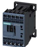
power contactor, AC-3e/AC-3, 12 A, 5.5 kW / 400 V, 3-pole, 220 V AC, 50/60 Hz, auxiliary contacts: 1 NO, spring-loaded terminal, size: S00
