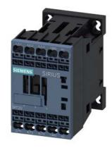
power contactor, AC-3e/AC-3, 12 A, 5.5 kW / 400 V, 3-pole, 230 V AC, 50/60 Hz, auxiliary contacts: 1 NO, spring-loaded terminal, size: S00, upright mounting position
