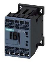
power contactor, AC-3e/AC-3, 12 A, 5.5 kW / 400 V, 3-pole, 220 V AC, 50 Hz / 240 V, 60 Hz, auxiliary contacts: 1 NC, spring-loaded terminal, size: S00
