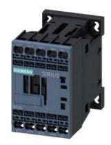
power contactor, AC-3e/AC-3, 12 A, 5.5 kW / 400 V, 3-pole, 400 V AC, 50/60 Hz, auxiliary contacts: 1 NO, spring-loaded terminal, size: S00
