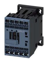
power contactor, AC-3e/AC-3, 12 A, 5.5 kW / 400 V, 3-pole, 24 V DC, auxiliary contacts: 1 NO, spring-loaded terminal, size: S00, communication-capable
