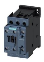
power contactor, AC-3e/AC-3, 32 A, 15 kW / 400 V, 3-pole, 230 V AC, 50/60 Hz, auxiliary contacts: 1 NO + 1 NC, screw terminal, size: S0, upright mounting position
