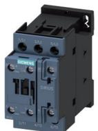
power contactor, AC-3e/AC-3, 32 A, 15 kW / 400 V, 3-pole, 208 V AC, 50/60 Hz, auxiliary contacts: 1 NO + 1 NC, screw terminal, size: S0, upright mounting position
