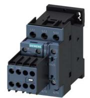
power contactor, AC-3e/AC-3, 32 A, 15 kW / 400 V, 3-pole, 220 V AC, 50/60 Hz, auxiliary contacts: 2 NO + 2 NC, screw terminal, size: S0, removable auxiliary switch
