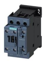
power contactor, AC-3e/AC-3, 32 A, 15 kW / 400 V, 3-pole, 230 V AC, 50 Hz, auxiliary contacts: 1 NO + 1 NC, screw terminal, size: S0  $\,$
