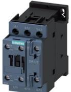
power contactor, AC-3e/AC-3, 32 A, 15 kW / 400 V, 3-pole, 220 V AC, 50 Hz / 240 V, 60 Hz, auxiliary contacts: 1 NO + 1 NC, screw terminal, size: S0
