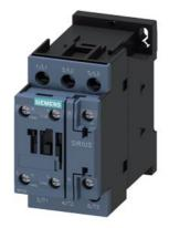
power contactor, AC-3e/AC-3, 32 A, 15 kW / 400 V, 3-pole, 380 V AC, 50/60 Hz, auxiliary contacts: 1 NO + 1 NC, screw terminal, size: S0  $\,$
