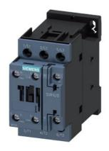
power contactor, AC-3e/AC-3, 32 A, 15 kW / 400 V, 3-pole, 400 V AC, 50 Hz, auxiliary contacts: 1 NO + 1 NC, screw terminal, size: S0  $\,$
