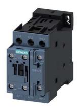
power contactor, AC-3e/AC-3, 32 A, 15 kW / 400 V, 3-pole, 24 V DC, auxiliary contacts: 1 NO + 1 NC, screw terminal, size: S0, communication-capable
