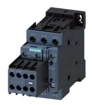
power contactor, AC-3e/AC-3, 32 A, 15 kW / 400 V, 3-pole, 24 V DC, auxiliary contacts: 2 NO + 2 NC, screw terminal, size: S0, removable auxiliary switch
