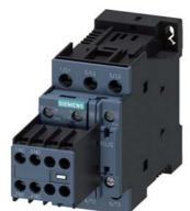
power contactor, AC-3e/AC-3, 32 A, 15 kW / 400 V, 3-pole, 110 V DC, auxiliary contacts: 2 NO + 2 NC, screw terminal, size: S0, removable auxiliary switch
