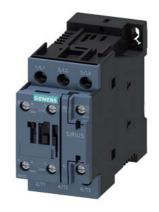
power contactor, AC-3e/AC-3, 32 A, 15 kW / 400 V, 3-pole, 72 V DC, auxiliary contacts: 1 NO + 1 NC, screw terminal, size: S0  $\,$
